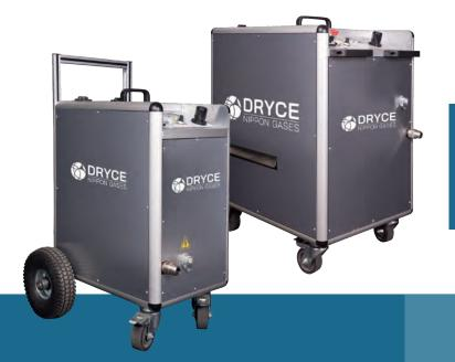
By appropriately selecting the nozzle model and dialing up or down the pressure, you can modulate the intensity of the cleaning jet, according to actual needs.
